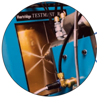
Figure 1 Spray pattern testing with the EUI Poptest HK862
