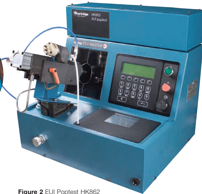
Figure 2 EUI Poptest HK862 fitted to a Testmaster 3 HH701
