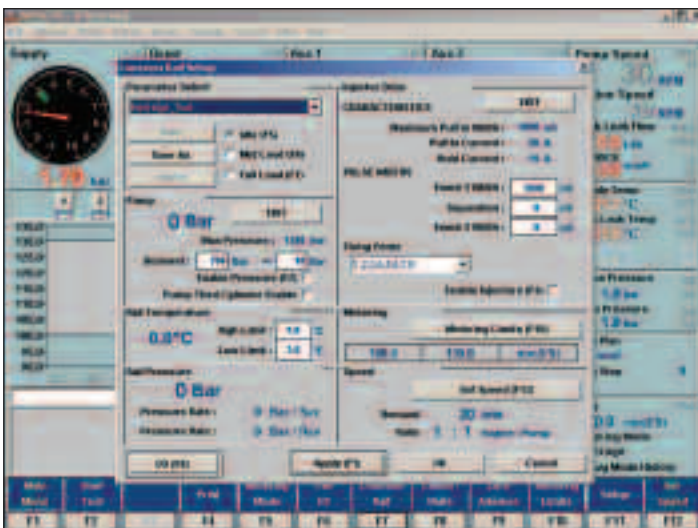
Figure 1 AVM2-PC Test Stand, Common Rail control screen display
